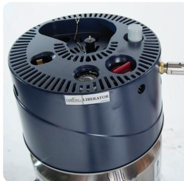
Clean the reservoir and portable unit fill connections to remove moisture and other contaminants with a lint free cloth.
