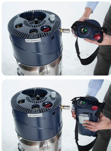
If the portable unit freezes to the reservoir while filling, simply close the vent valve handle and leave it attached. Once the fill connectors have thawed, the units can then be easily disengaged.
