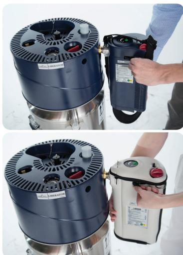
Begin filling the portable unit by simply pulling its black vent valve handle into its open position while continuing to apply pressure on the portable unit to maintain its connection.
