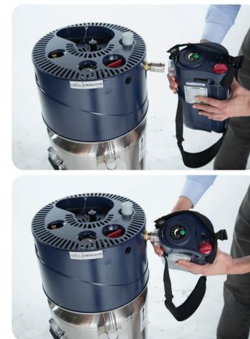
Position the portable unit so that the indentation in the left of the portable is aligned with the fill connector on the side of the reservoir. Connect the portable with the reservoir and turn the portable counter clockwise to engage it with the reservoir. Once the portable unit is engaged with the reservoir, return it to its upright position. The portable unit can now be filled.
